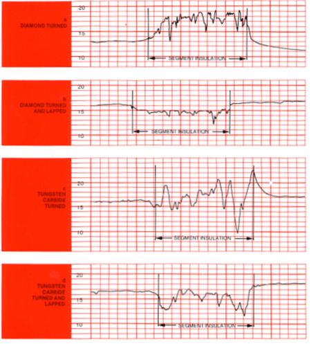
Scale: Vertical 40 micro inches per division COMPARISON OF DIFFERENT SURFACE FINISHES
